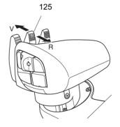
When the limit position for the operation has been reached (there will be a noise from the pressure relief valve) release the lever. The lever will revert automatically to neutral.
