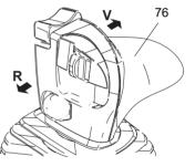
When the limit position for the operation has been reached (there will be a noise from the pressure relief valve) release the lever. The lever will revert automatically to neutral.
