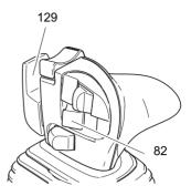
• Pull the (129) button while at the same time pressing the (82) button, the forks will move together.
