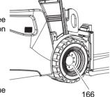
When using pneumatic tyres check the air pressure, for the air pressure see "Tyre type" on page 28
