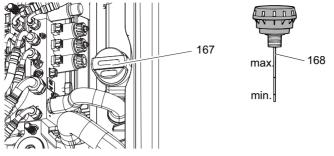
Checking the hydraulic oil level and adding hydraulic oil
