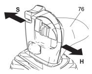
Hen the limit position for the operation has been reached (there will be a noise from the pressure relief valve) release the lever. The lever will revert automatically to neutral.
