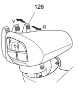
Hen the limit position for the operation has been reached (there will be a noise from the pressure relief valve) release the lever. The lever will revert automatically to neutral.
